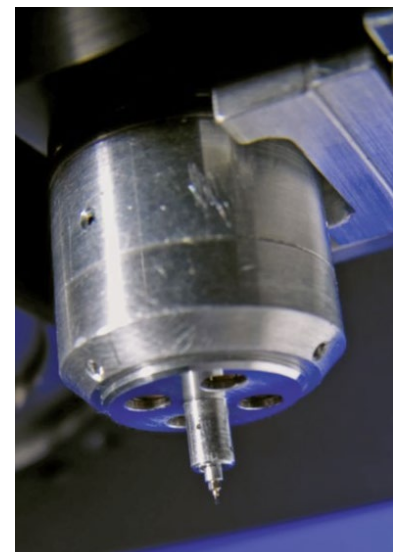
Figure 3. DCMII head with Berkovich tip installed.
